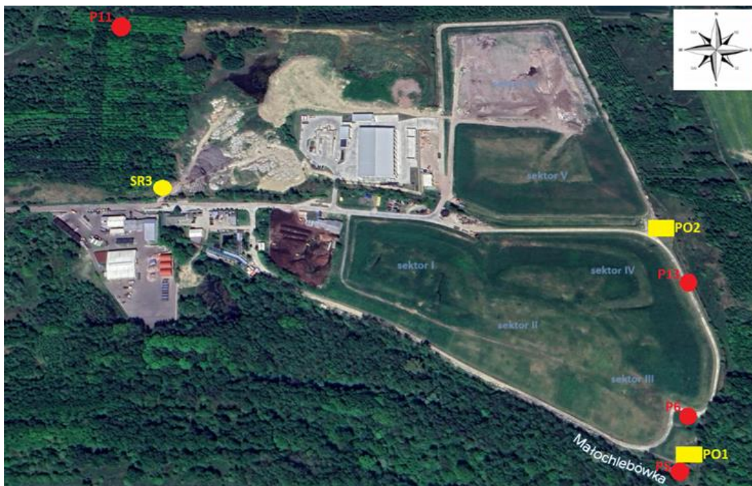
Figure 1. Location of groundwater and leachate testing points in the area of the landfill (northeastern Małopolska, southern Poland)
