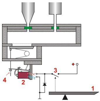
Figure 8. Scheme of electromagnetic key action in conjunction with pallet windchest 1 - key, 2 - electromagnet, 3 - switch, 4 - valve tie bar
