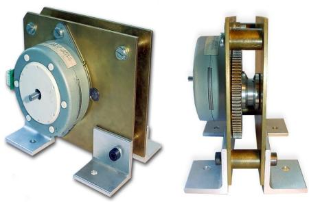
Figure 11. The prototype of stepper-motor module for controlling the valves in the tone windchest
