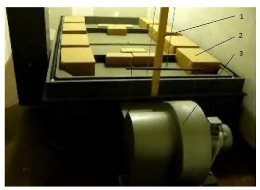
Figure 7. View of the organ bellows 1 - Bracket of the control gear for filling the bellows (throttle), <math>2 - weights, 3 - blower
