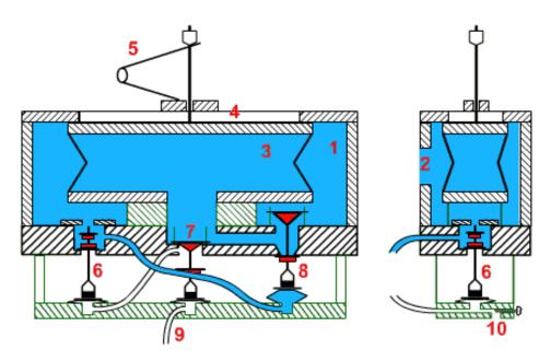
Figure 9. Tremulant operating scheme
