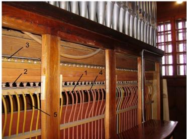
Figure 4. Pneumatic key action in no longer existing organ of St. Roch's Church in Nowy Sącz, Poland, made by the organ-builder Stanisław Aleksander of Rdziostów near Nowy Sącz 1 – supply tube, 2 – tappet-equipped bellows powered by low pressure air, 3 – tappet-equipped bellows powered by higher pressure air, 4 – adjustment screw, 5 – main bellow / tank
