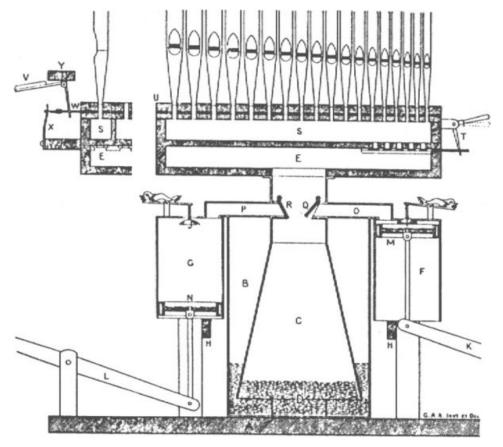
Figure 1. Water organs of Ctesibius - cross section
