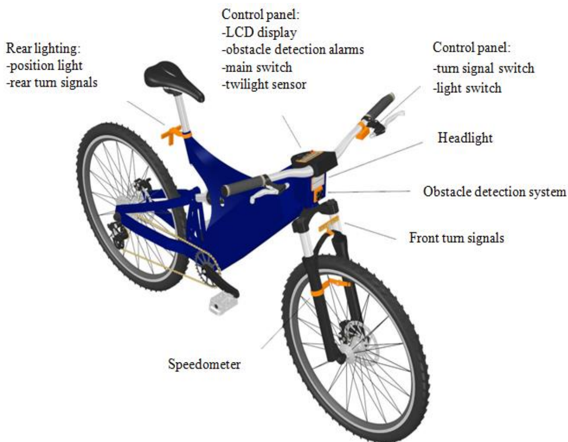
Figure 12. Layout of electronic systems
