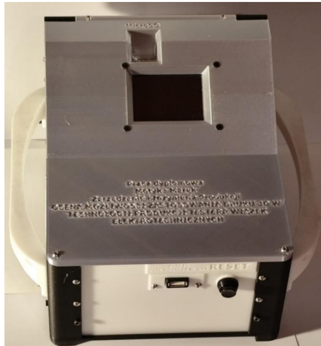
Figure 6. View of the assembled prototype of the wire harness tester
